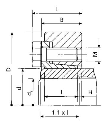
B mm = 29.5 d H8 mm = 68 D mm = 115.0 ds mm = 50 F kN torque = 76 H = 3.5 I mm = 24.5
